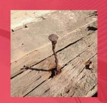
Galvanized nails/screws in pressure treated wood → prevents
